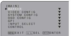
**3** Use the HD ZOOM/v button and BLUE/A button to align the cursor with the item to be changed, and press the FUNCTION/ENTER button. The setting is now displayed in green.
